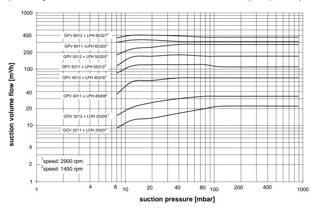
For the suction volume flow the tolerance is 10 %.
