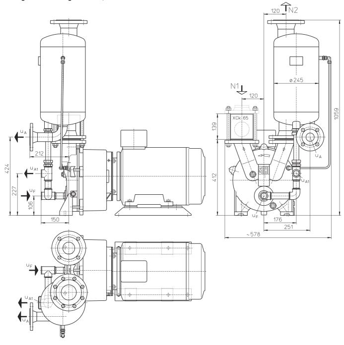
N 1 = gas inlet DN 65 N 2 = gas outlet DN 80  $u_A = liquid drain DN 40$  $u_{A1} = liquid drain G 1$
