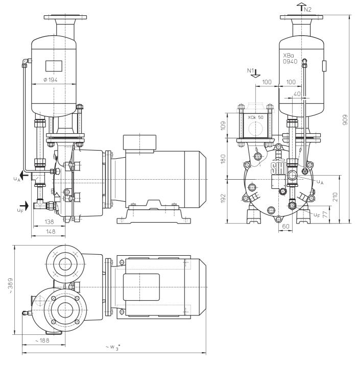
gas inlet DN 50 gas outlet DN 65 = liquid drain G 1
