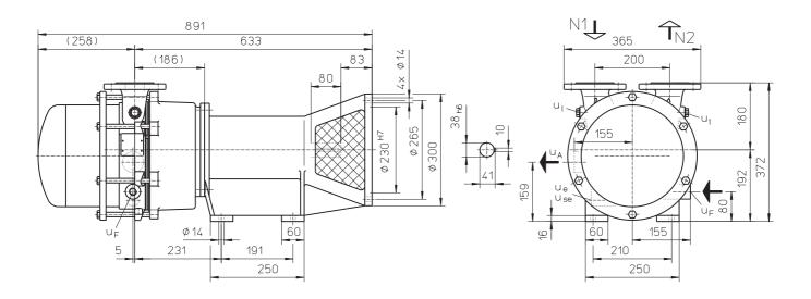
N 1 = gas inlet DN 50 N 2 = gas outlet DN 50  $u_A$  = liquid drain G 1 $\frac{1}{4}$
