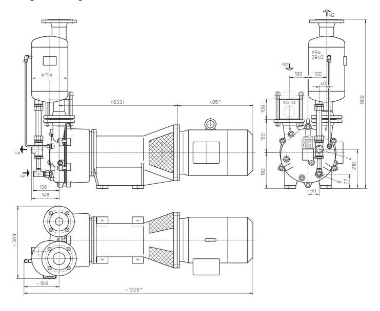
N 1 = gas inlet DN 50 = gas outlet DN 65 = liquid drain G 1
