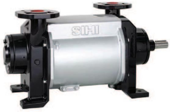
The Sterling SIHI liquid ring compressors LPH 40106 and LPH 40411 are one stage. They can be used without modification as vacuum pumps up to a suction pressure of 150 mbar (for more information see Catalogue Part LI 2).
