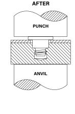
Shown with blind mounting hole. Can also be used with a through hole.
