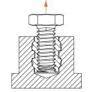
**Pullout** is the force required to pull the insert from the sheet.
