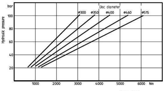
NOTE: For holding duty the above torque values to be reduced by 50 %
