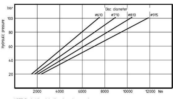
NOTE: For holding duty the above torque values to be reduced by 50 %
